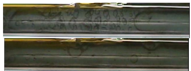
Fig. 3 Flow behavior in 1g (top) and micro-g (bottom) under G = 35 \text{ kg/m}^2\text{s} , q = 14 \text{ kW/m}^2 at segment 2.
