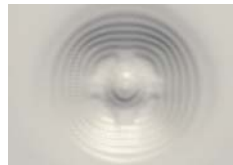
Figure 3: surface deflection in the heater region of a water film resting on a horizontal plane
