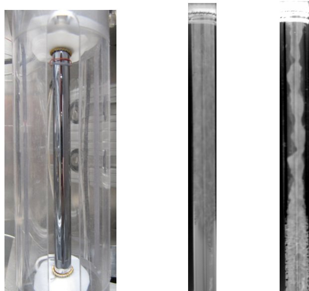
Figure 1: Photograph of silicon tube (left) and IR image of bubble flow in high-g (middle) and inverted annular flow in low-g (right).
