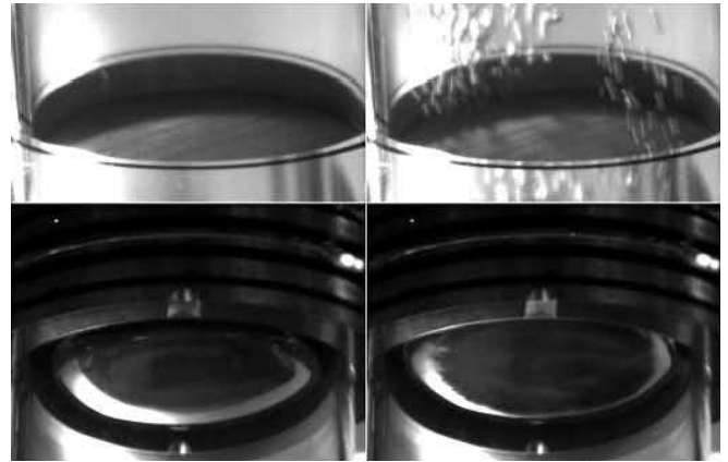
Figure 2: Experimental observation of the trapped bubble as it breaks through the porous screen at a sufficiently high liquid flow rate.
